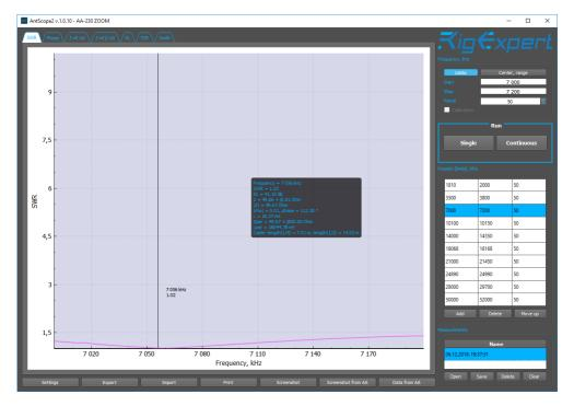
Type your Frequenz in the **Start** field and in the **Stop** field set your end Frequenz klik on **Add** and your setup is saved
