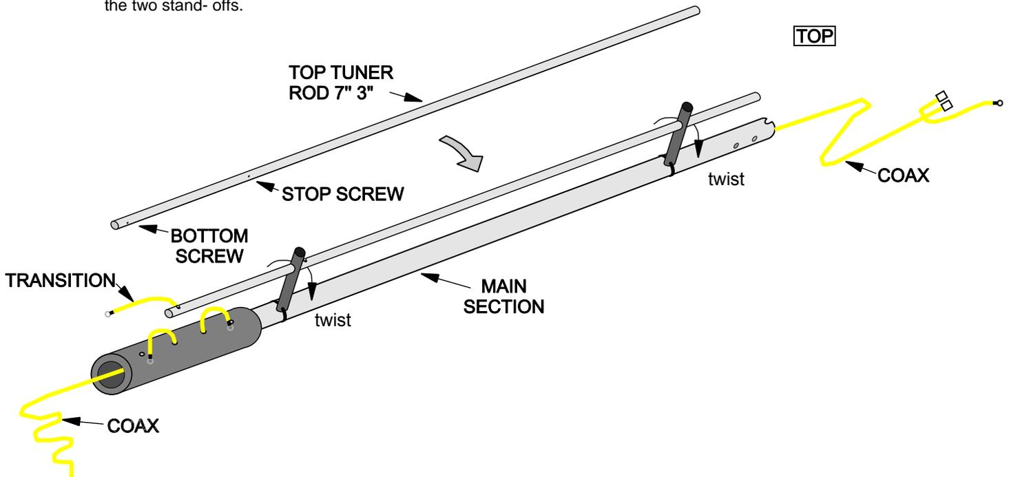
2) A sheet-metal screw is used as a stop screw, to keep this rod from sliding downward. Make sure the stop hole is above the stand-off. Insert a screw and lock washer in the stop hole, and tighten.
