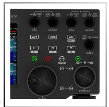
touch screen display bypassing the complexity of multi-function buttons and multi-level menus found on most transceivers. Like modern phones and tablets, capacitive touch control is provided on the large LCD display for intuitive pan, zoom, tune, and menu operation.
